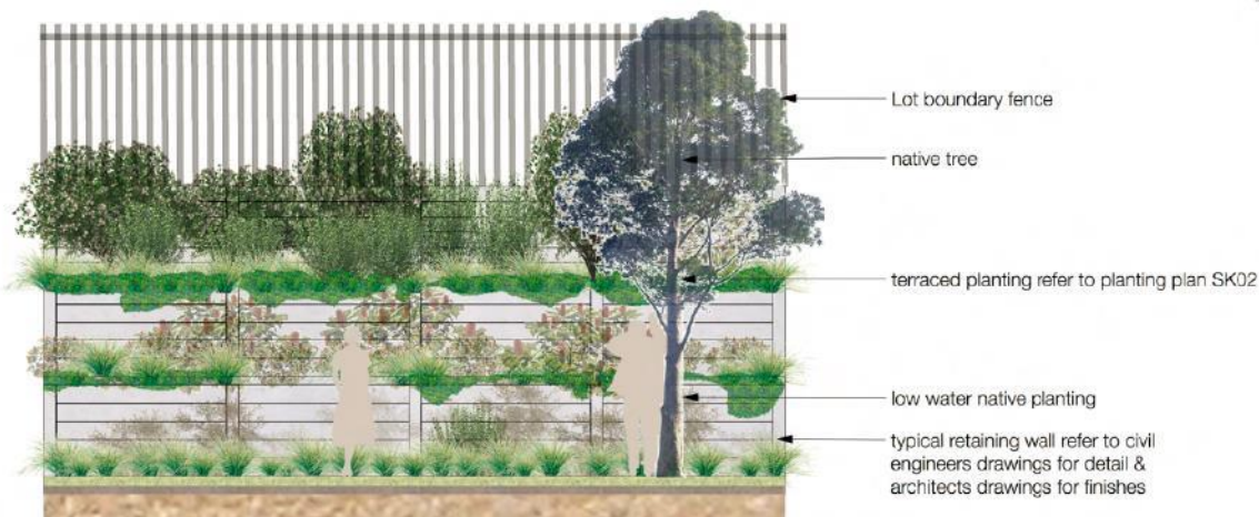
Figure 12 Typical Elevation of a 3 tier retaining wall
